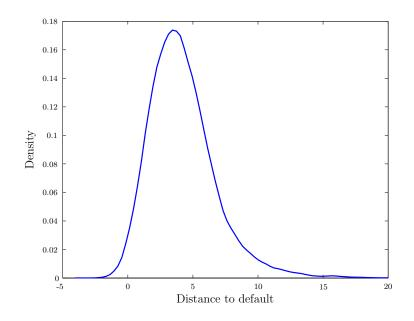
Figure IA.II. DTD population density. Population density estimate of distance to default for 402,434 firm-months between January 1979 and March 2004. The estimate was obtained by applying a Gaussian kernel smoother (bandwidth equal to 0.2) to the empirical distribution.
