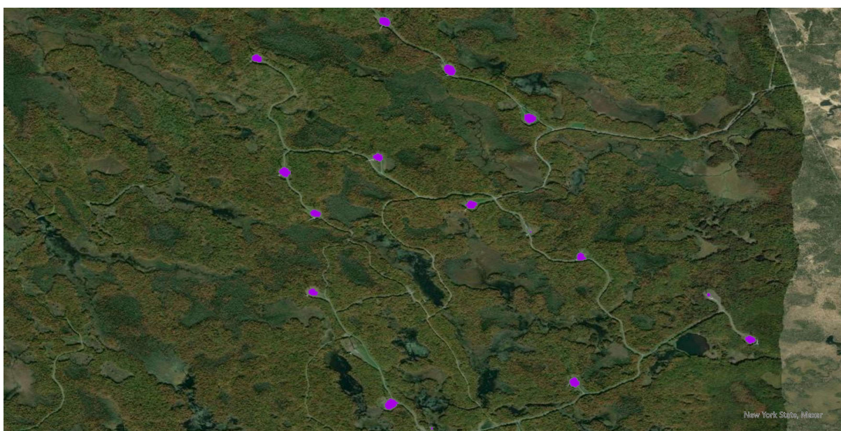
Figure IA I 4: These figures illustrate the identification of a wind plant footprint using Sentinel-2 satellite data. The plant is the Roaring Brook Wind Farm in New York State, U.S., with a capacity of 79.7 MW. The top picture shows the original satellite image. The bottom picture illustrates the plant detection algorithm, with the wind turbines colored in purple.
