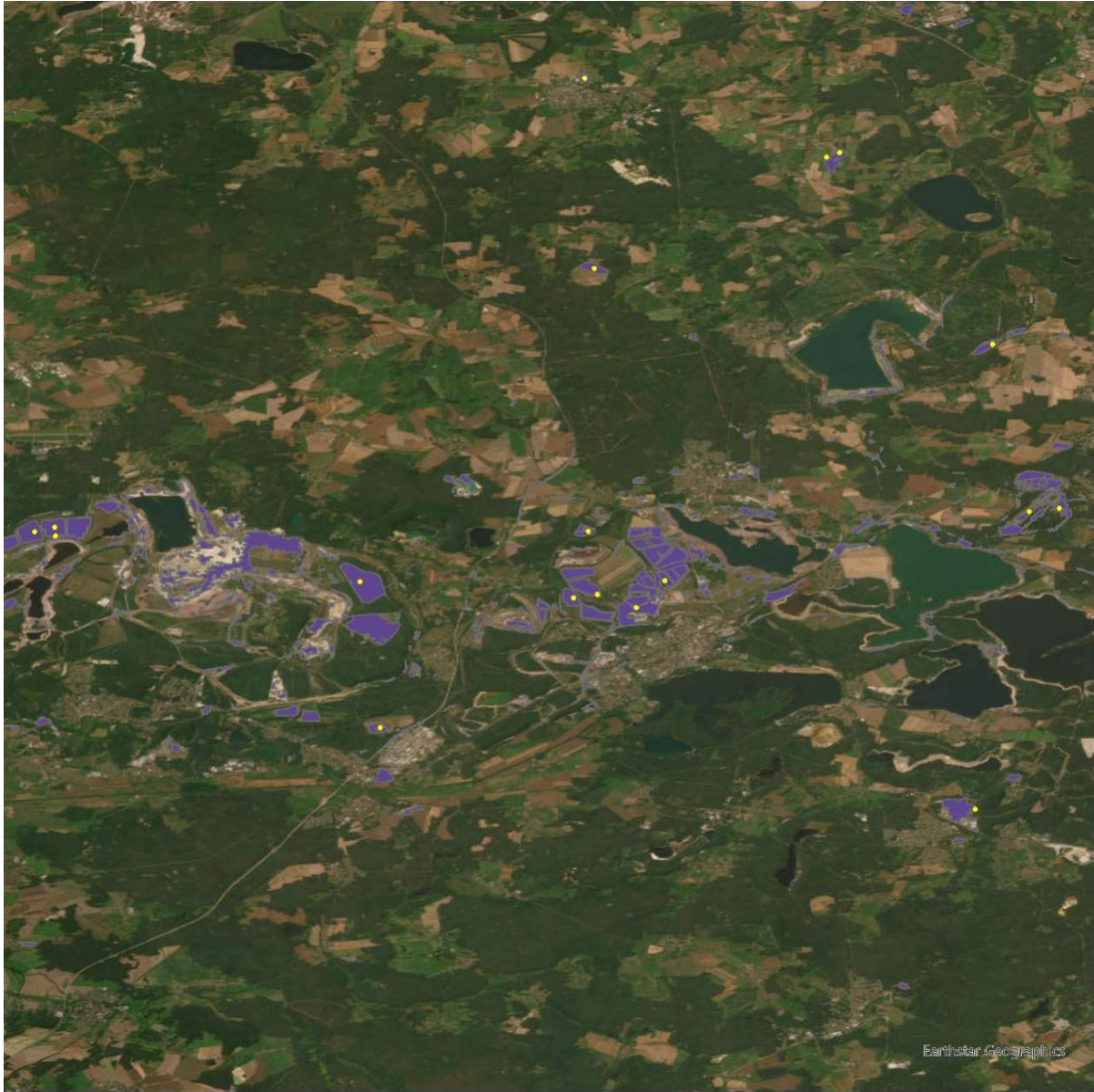
Figure IA I 3: This figure shows the detected solar farm footprints near Königsberg, Germany. This example illustrates the methodology for handling clusters of plants, where total land use is calculated for closely-sited facilities and then allocated to individual plants based on their capacity.
